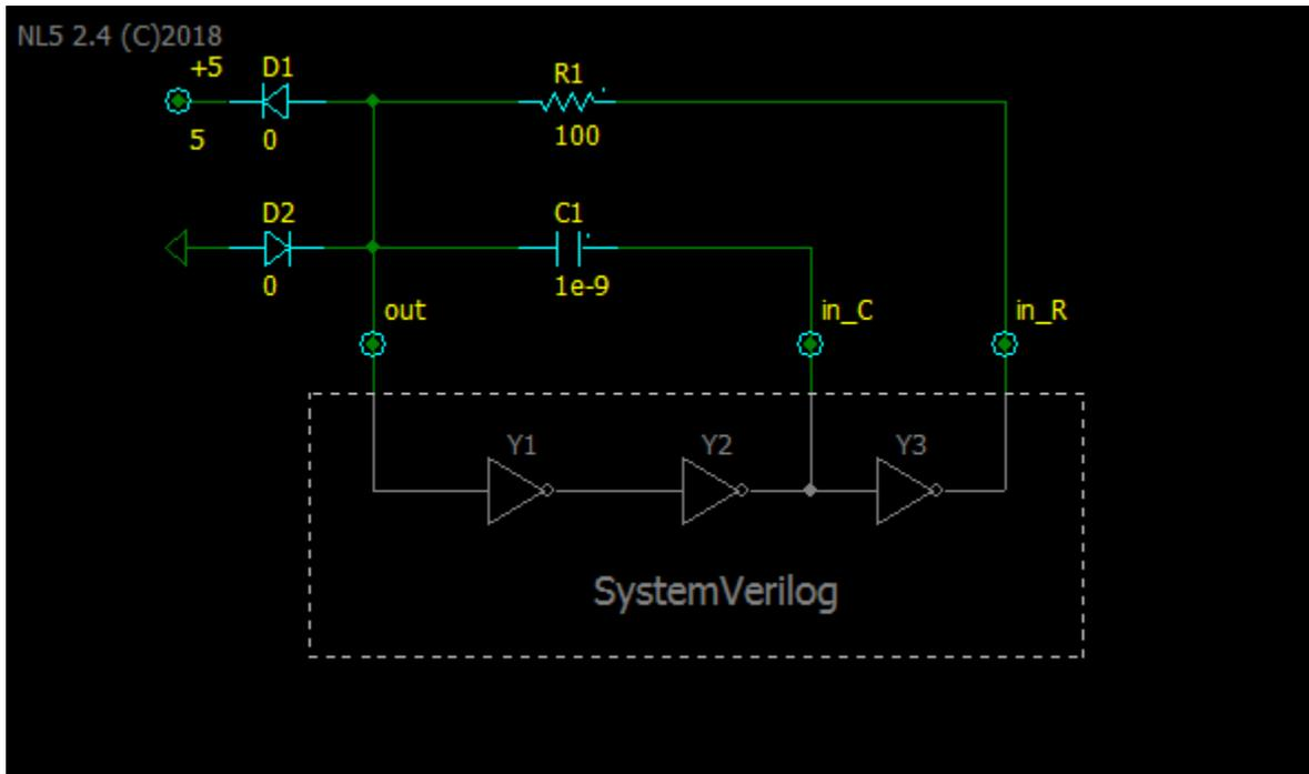
Digital part (Y1, Y2, Y3) of the circuit is disabled, since it will be simulated by SystemVerilog. Labels “out”, “in\_C”, and “in\_R” are used for passing signals between analog and digital parts.
