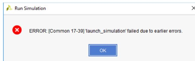
Click “OK” two times. This step is required in order to force Vivado to create simulation directory, and then copy required nl5 demo files into that directory.
