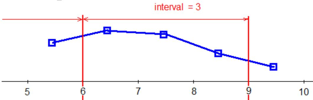
Now, all the data of the new calculated interval between  $t = 6s$  and  $t = 9s$  can be retrieved using interpolation.
