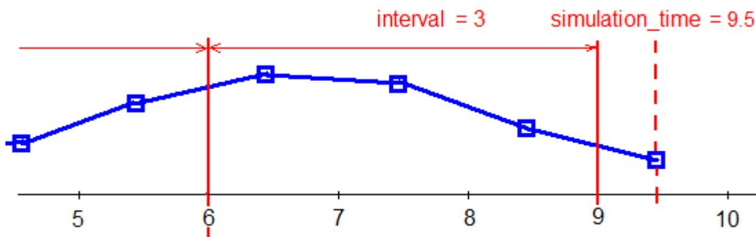
Using `NL5_Simulate` function provides the best simulation performance. It won't decrease simulation step at the end of current linear range, so that there is no need to restore the step back as simulation continues. Thus, the simulation will be performed in the fastest manner, regardless of simulation interruptions.
